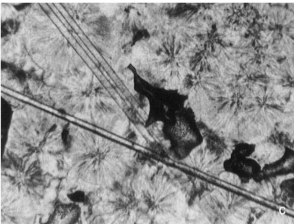
Figure 6 Micrographs of polypropylene crystallization in the presence of SGF, in a matrix based on 95/5 PP/LDPE blend, at 403 K ( \times 125 )
